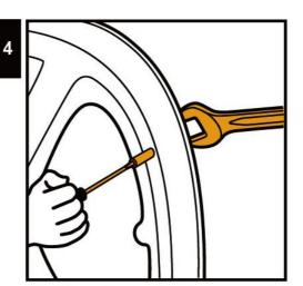
Tighten the valve by wrench and screw it ( Torque value must be  $\geq$  4Nm)
