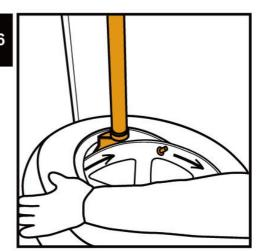
Install the tire from left side of the valve clockwise direction, avoid tire bead hits valve and sensor.
