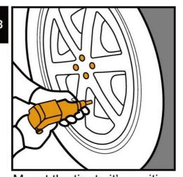
Mount the tire to it's position. 依照輪胎位置將已裝好無線傳感器之輪胎分別裝回原位
