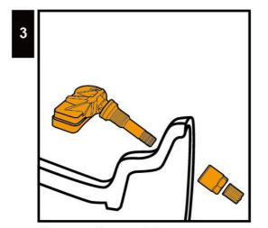
Sensor Assemble 無線胎壓傳感器安裝
