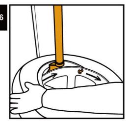
Install the tire from left side of the valve clockwise direction, avoid tire bead hits valve and sensor.
