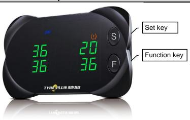
The driver can follow the steps to adjust the system of pre-loaded values Notice: the system has been pre-set with alert figures. If the driver wants to change the figure, then follow the professional tire technician's instruction.
