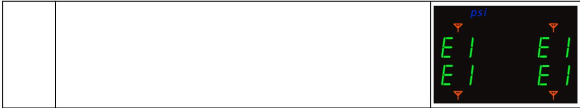
**Note** when display unite shows E1 or E2, place any wireless devices (cell phone, etc) further away from display unit or locate a qualified tire service center to correct the issue.
