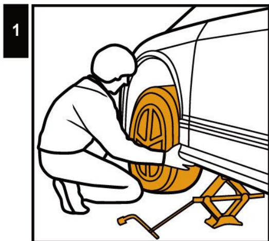
1 Jack up the car and de-mount the tire.
